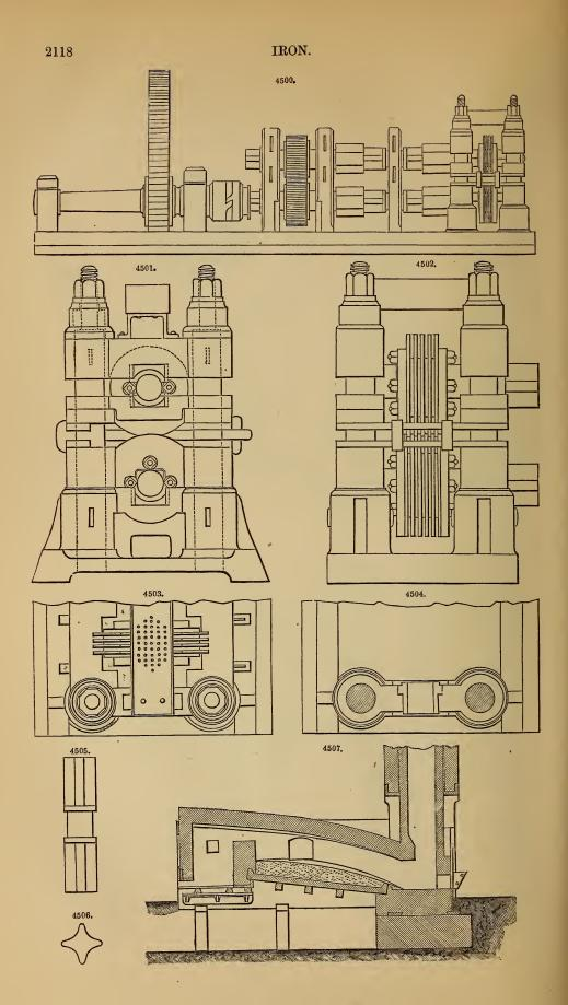
to the rolls. The drawing out, charging a fresh heat, and repairing the bottom, will average six-teen minutes a heat. Piles of this size weigh about 4 cwt. each. At this rate, a heating furnace will work thirty-six piles in the twelve hours, or 83 tons of iron a week.
